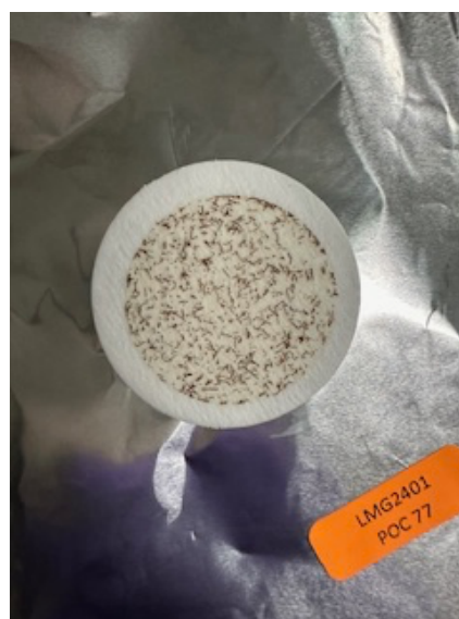
Figure 3. Filter for POC analysis from 50 m sediment trap showing krill fecal pellets. Photo by Zephyr Girard.
