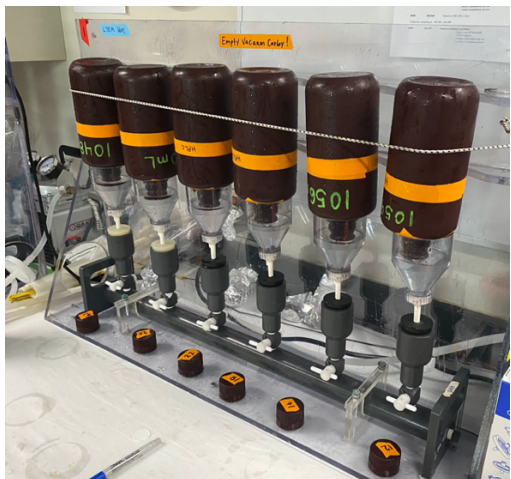
Figure 4. Filtering water for High Performance Liquid Chromatography (HPLC) pigment measurements. For phytoplankton community structure. Photo by Jake Gessay.
